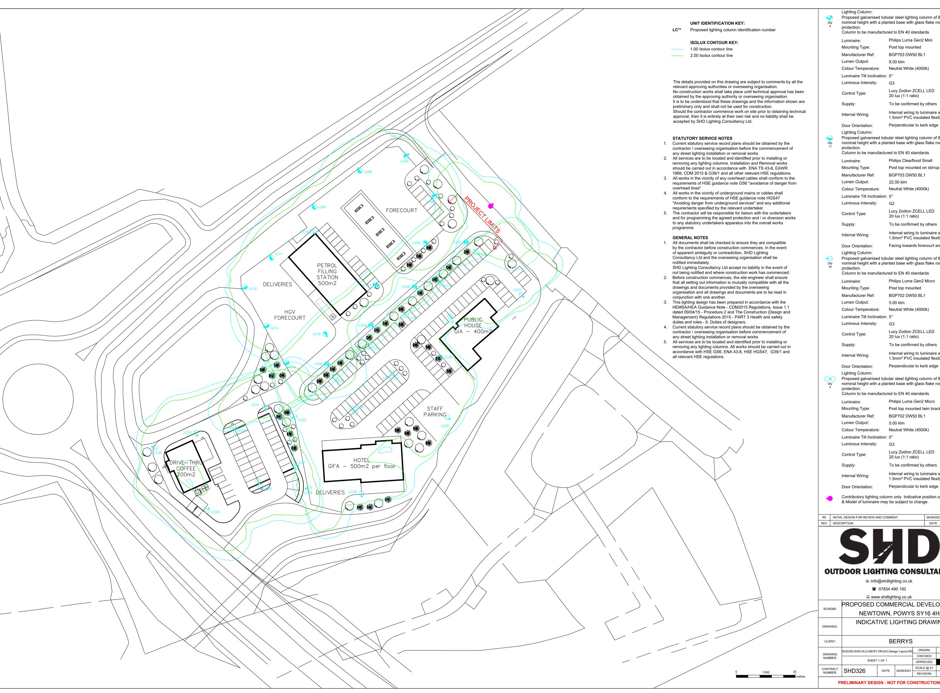
Proposed galvanised tubular steel lighting column of 8.0 metre nominal height with a planted base with glass flake root
